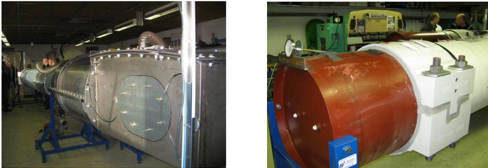
Figure 13 Full scale testing of sealing, left saddle and shroud, right cable band and transition at band
