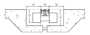
of these two movements should be used to select the appropriate Steelflex<sup>®</sup> Modular Expansion Joint System.
