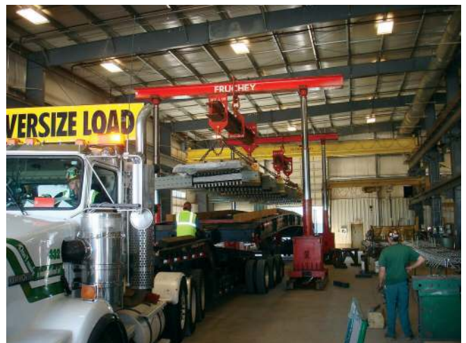
Expansion Joint being loaded onto truck.
