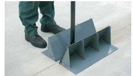
Trough & Tapper™ for seals from 1-1/4 to 4 inches nominal width
